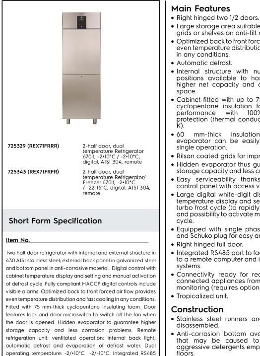
Large storage area suitable to contain 2/1 GN grids or shelves on anti-tilt runners. Optimized back to front forced air flow provide even temperature distribution and fast cooling in any conditions. Automatic defrost. Internal structure with numerous charging
